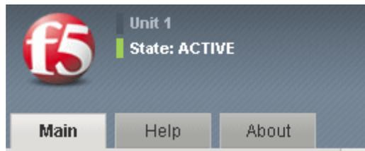
*Figure 4.1 Cluster status indicator in the Configuration utility*
