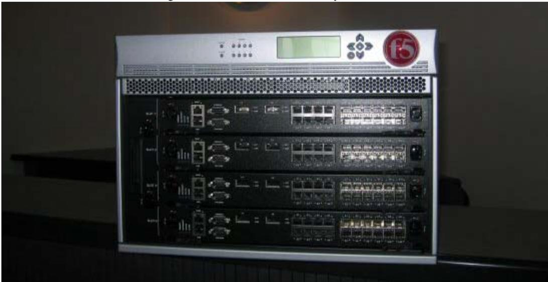
*Figure 1.1 A four-slot chassis with four blades installed*
